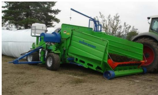
Fig. 1. Press for filling polyethylene foil with fresh biomass
