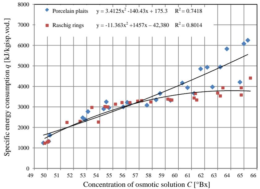
Fig. 7. Dependence of specific energy consumption  $q$  [kJ/kg<sub>isp.vod.</sub>] and concentration of osmotic solution  $C$  [°Bx] – Air temperature 70 °C
