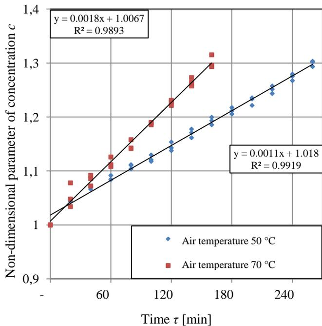
Fig. 4. Dependence of non-dimensional parameter of concentration  $c$  (ratio of current and initial concentration of solution) and duration of the process  $\tau$  - porcelain 'Raschig' rings
