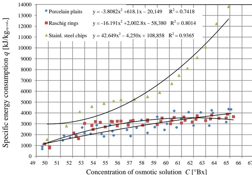
Fig. 6. Dependence of the specific energy consumption  $q$  [kJ/kg<sub>isp.vod.</sub>] and The concentration of osmotic solution  $C$  [°Bx] – The air temperature 50 °C
