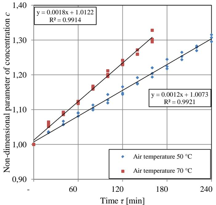
Fig. 5. Dependence of non-dimensional parameter of concentration  $c$  (ratio of current and initial concentration of solution) and duration of the process  $\tau$  - porcelain plait
