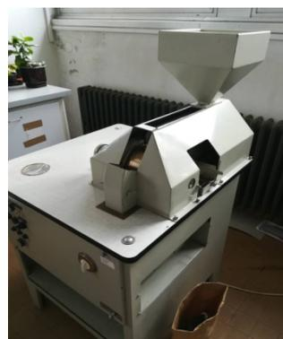
Fig. 5: Laboratory magnetic separator MCC Lilliput
