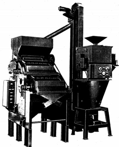
Figure 6: Emceka – Gompper magnetic cleaning machine
