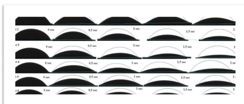
Figure 9. Change of contact angle CA from water drop on the pellet surface at different time intervals. The curved line symbolizes the initial water droplet profile
