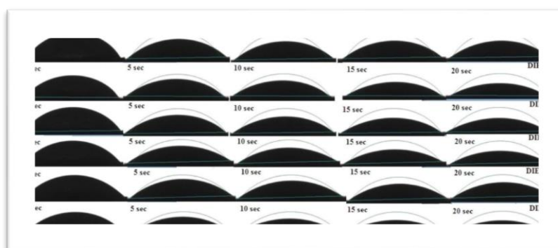
Figure 8. Change of contact angle (CA) from oil drop on the pellet surface at different time intervals. The curved line symbolizes the initial oil drop profile
