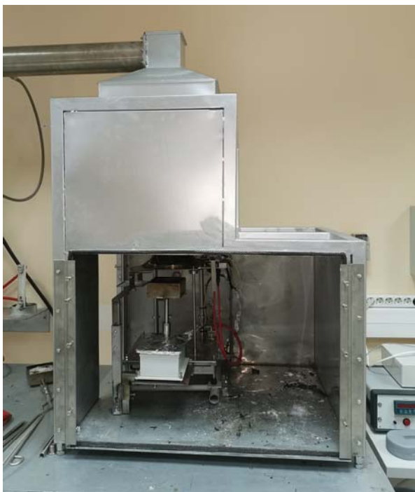
Figure 2. Mass loss calorimeter inside the specially designed fume cupboard
