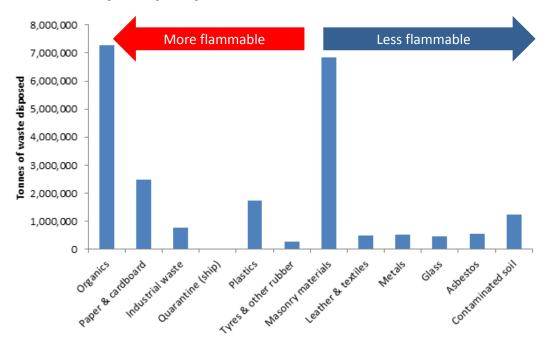
**Figure 1.** *Flammability of different waste types* [3]
