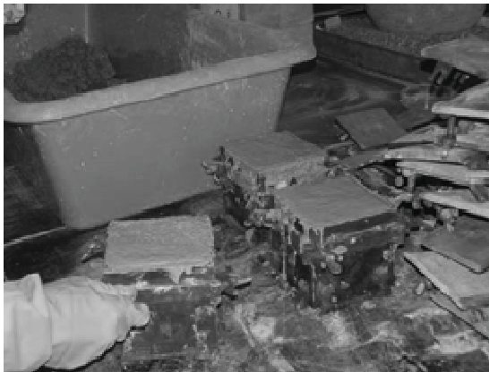
Slika 8. Priprema uzoraka betona Figure 8. Preparation of concrete samples
