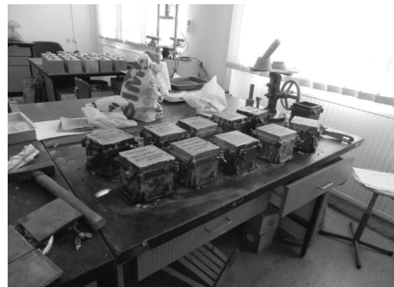
Slika 8. Priprema uzoraka betona Figure 8. Preparation of concrete samples
