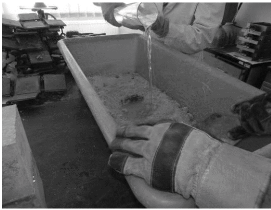
Slika 7. Priprema uzoraka betona Figure 7. Preparation of concrete samples
