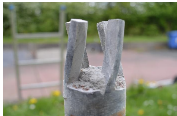
Figure 14. Excessive bending of strips
