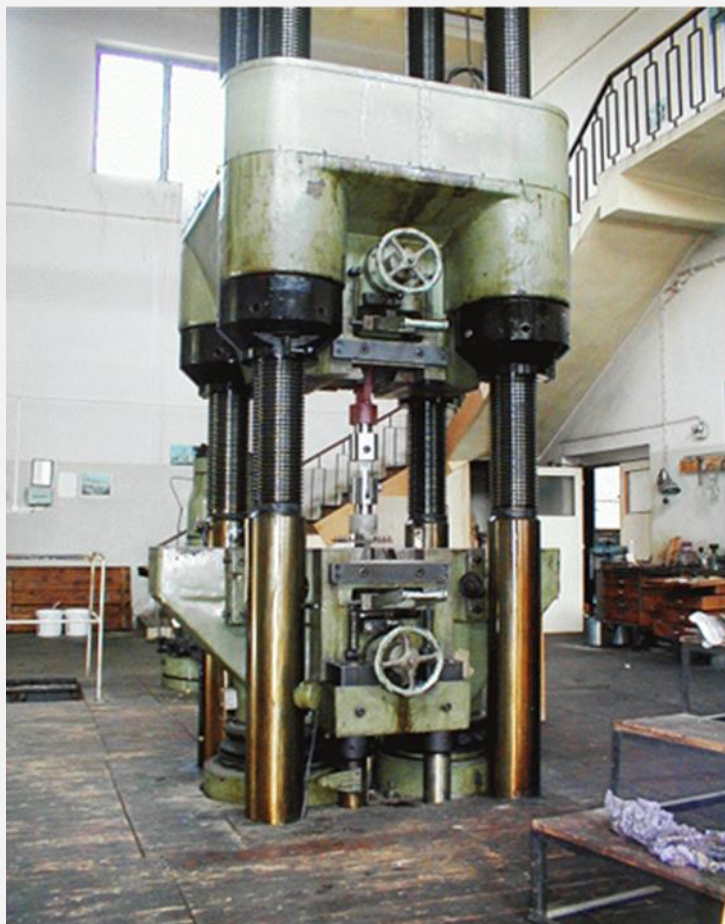
Fig. 7. Pulsator with loading capacity of 6000 kN adopted
