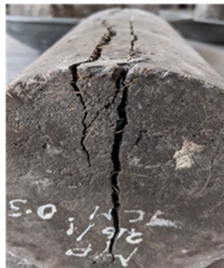
Figure 10. Failure pattern of fiber reinforced cylinder specimen
