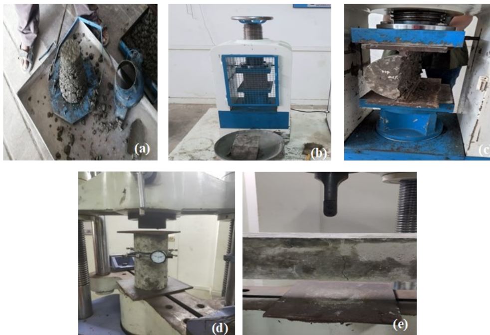
Figure 6. Experimental test procedure for FTPF reinforced concrete(a) Slump test (b) Compression test (c) Splitting tensile strength test (d) Modulus of elasticity (e) Flexural strength
