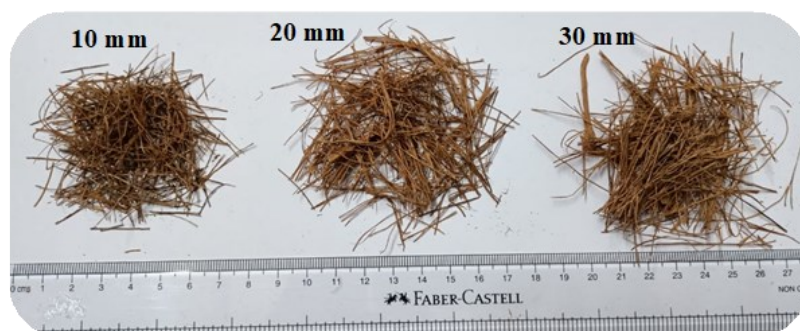
Figure 5. Cut fish tail palm fibers of different length
