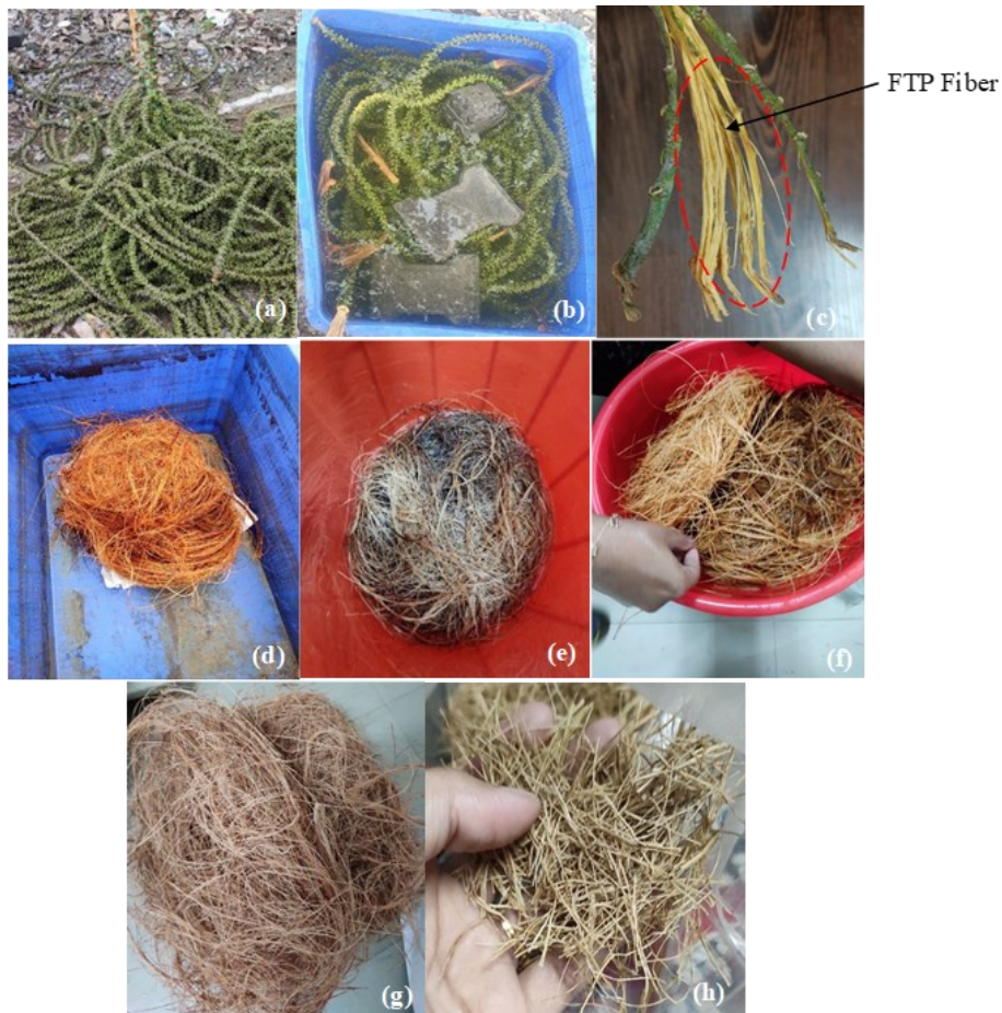
(a) Raw fibers from palm tree (b) Fiber stems immersed in water (c) Beaten fibers to remove outer skin (d) Fibers extracted from outer skin (e) Silane chemical treatment (f) Fibers washed in ethanol (g) Oven dried fibers (h) Fibers cut into different length
