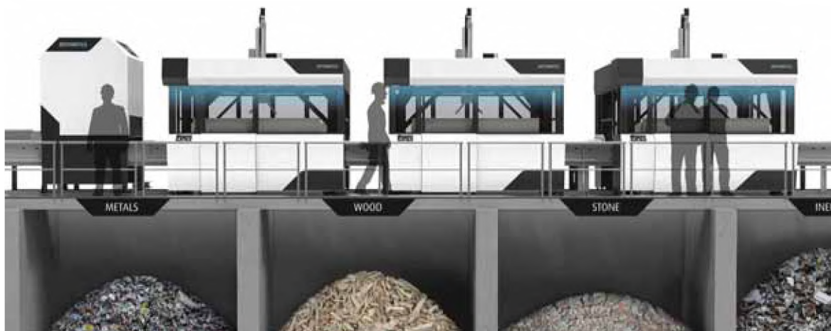
Fig. 3. ZenRobotics technology heavy picker sorting line [23]
