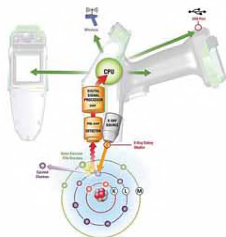
Fig. 11. The X-ray instrument emits energy which changes the electrons orbitals [122]
