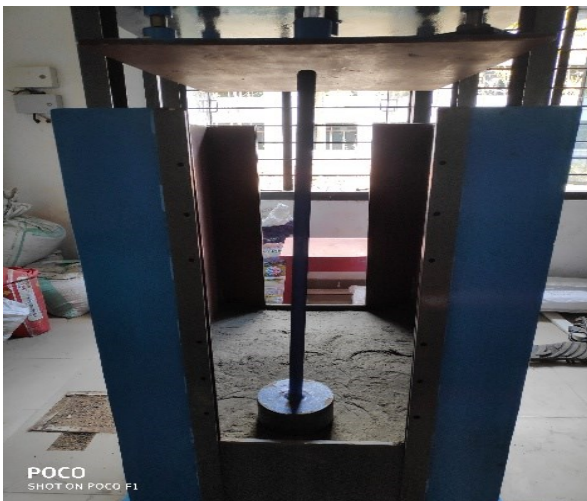
Figure 8. Compacted a dense M-Sand bed
