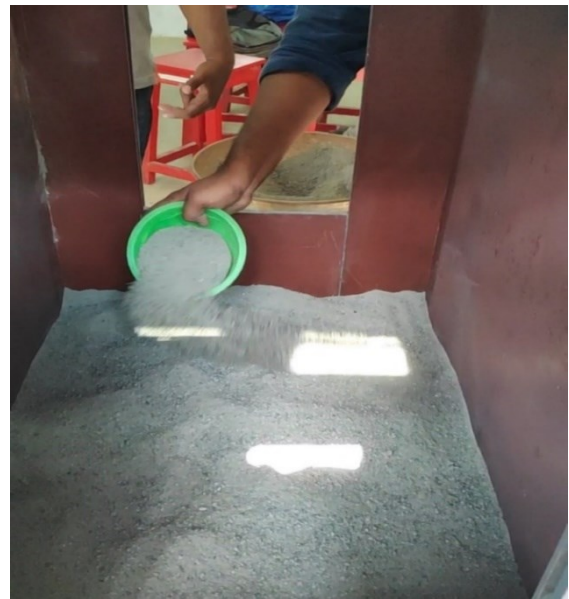
Figure 9. Filling of loose M-Sand bed
