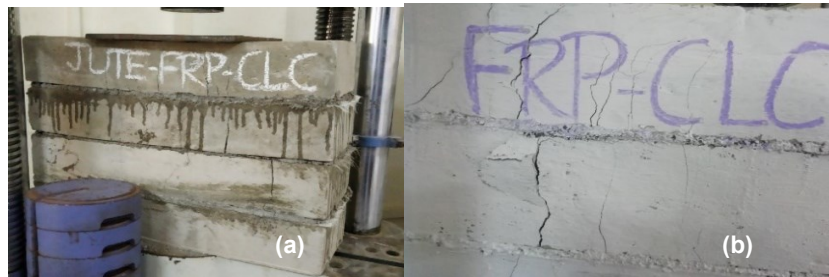
Figure 3. Crack pattern in masonry unit without fibre and with natural fibre
