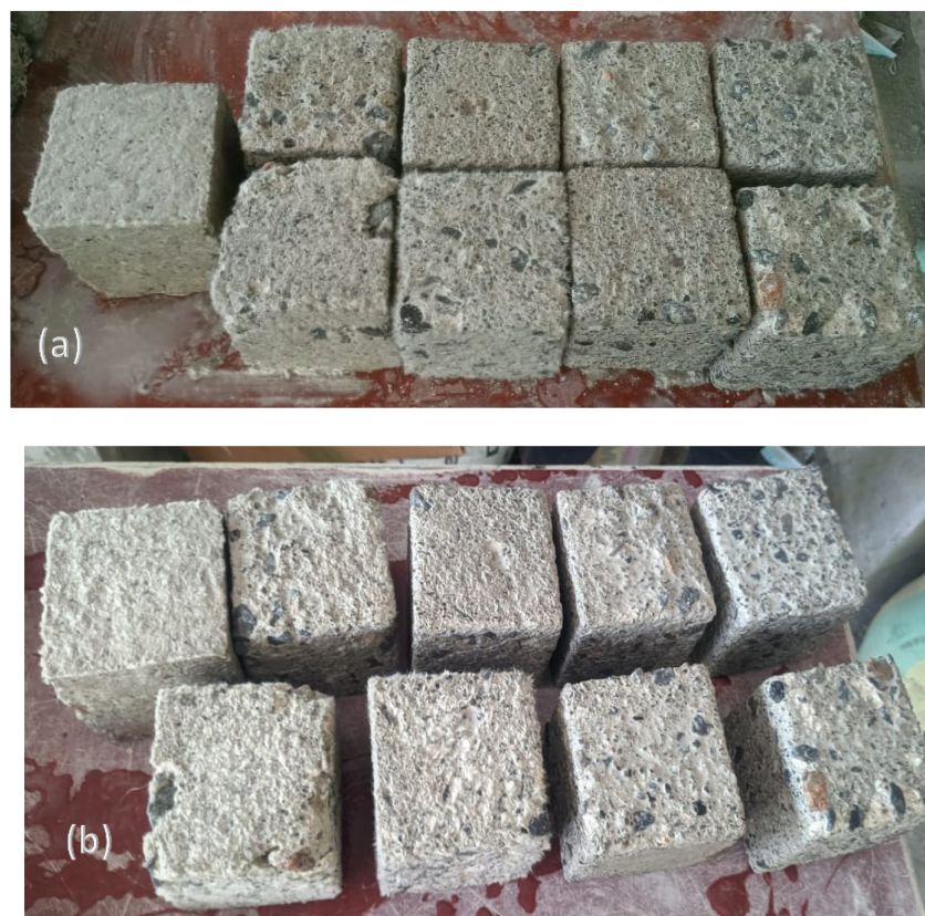
Figure 15. Acid attack specimen after (a) 7 days and (b) 14 days
