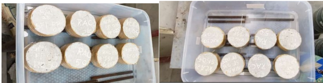
Figure 5. Water absorption test arrangement for control Mix, RAC and HYFRAC specimen
