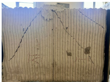
Figure 15. The failure mechanism of the segmental beam in 3-point test – front side
