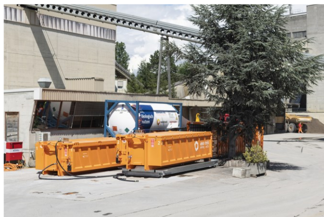
Figure 6. Industrial mineral carbonation plant (two reactor containers, \text{CO}_2 storage tank and centre for the process control) [90]
