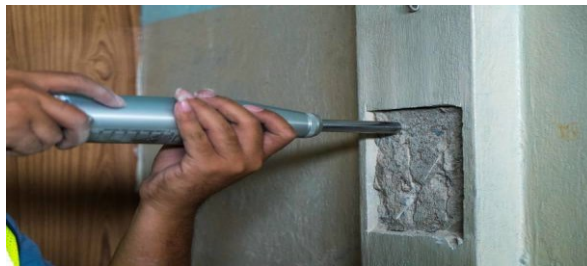
Fig. 2. Schmidt rebound hammer
