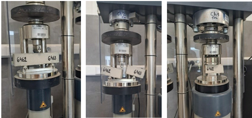
Figure 2. Testing of the mortar specimen
