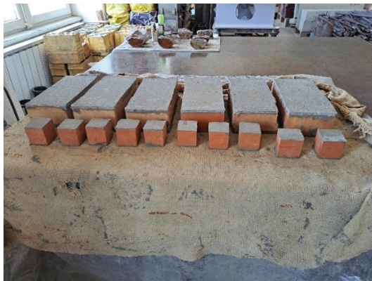
Figure 4. Preparation and testing of brick specimens
