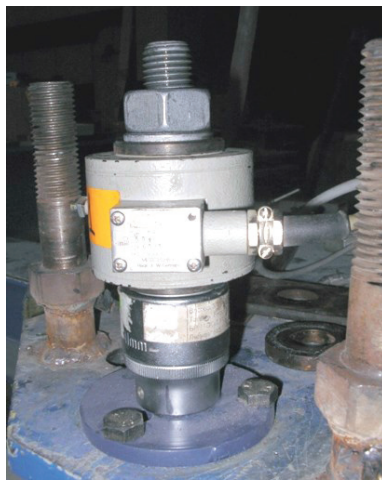
a) Setup for preload force measurements
