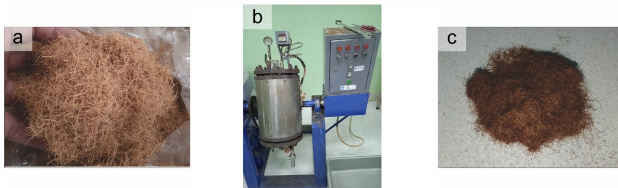
Figure 1. Preparation of hydrochar, a) coconut coir fiber (CCF), b) HTC rotary digester reactor, c) hydrochar
