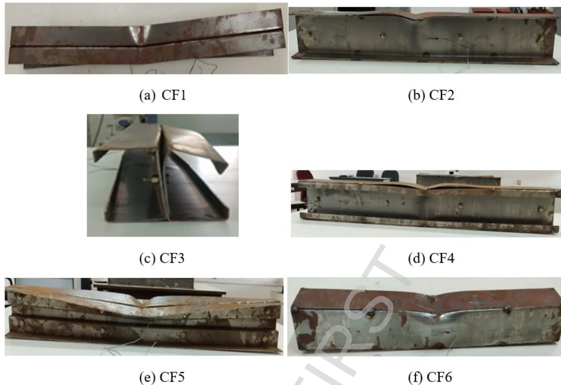
Figure 3. Tested CFS built-up beams
