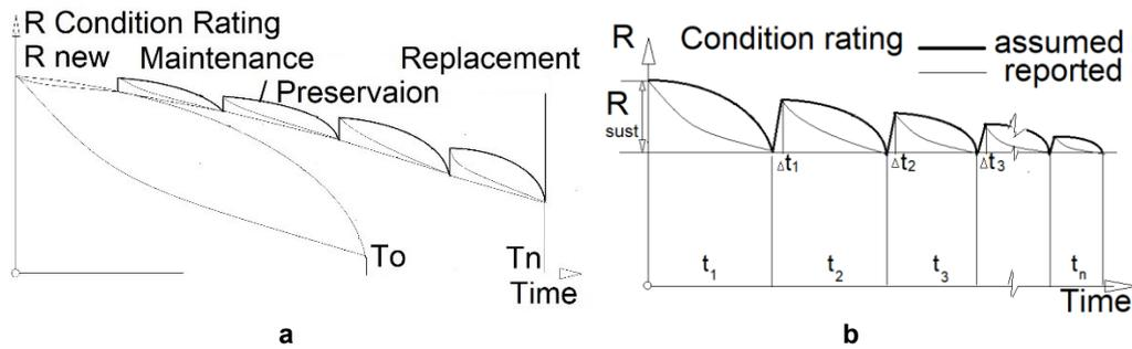
Figure 2. Hypothetical effect of periodic preservation interventions on extending the useful life of a bridge and a network
