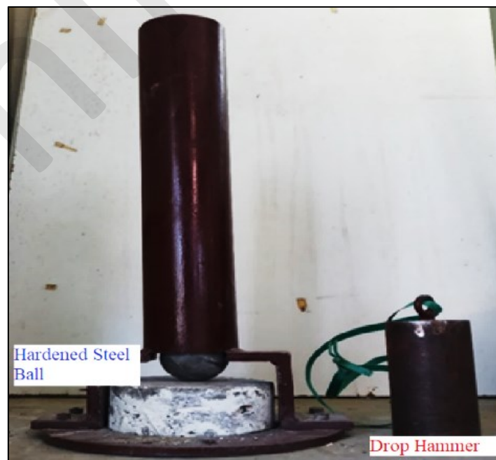
Figure 16. Test Setup for Drop Weight Impact Tester
