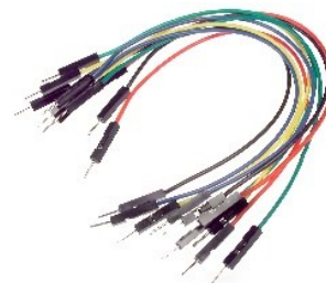
Figure 6: Jumper wires M-M
