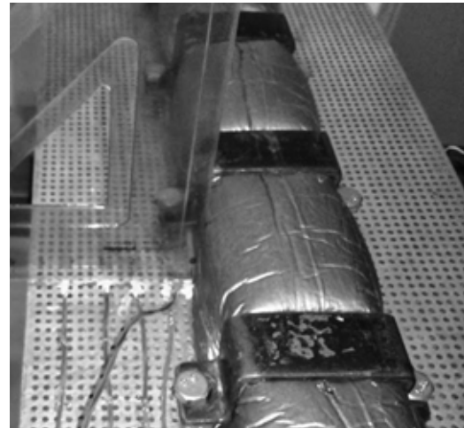
Figure 4. Thermocouples position on the perforated plate
