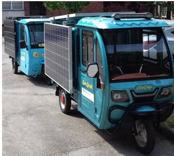
Figure 1. Solar cargo tricycle prototypes named SunSnail in Hungary
