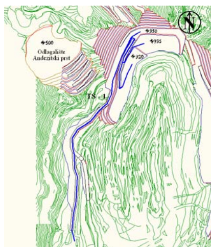
Figure 3 Mining layout of open pit South Mining District at the end of the second year with the presented transport route to the crushing plant (location A)
