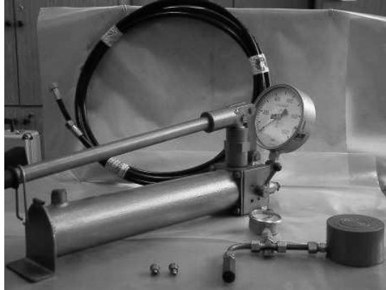
Figure 3 Measuring probe with additional tools for measuring the stress states
