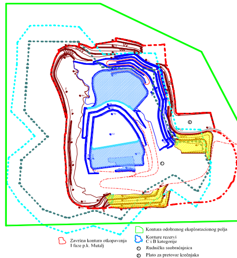
Figure 3 Plan of excavation in the IV year of the OP Mutalj - I stage
