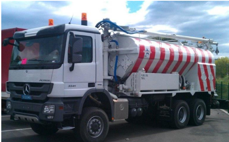
Figure 3 An-Fo vehicle for mechanized charging of boreholes
