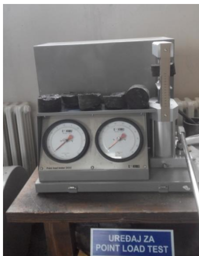
Figure 1 PLT device with prepared samples
