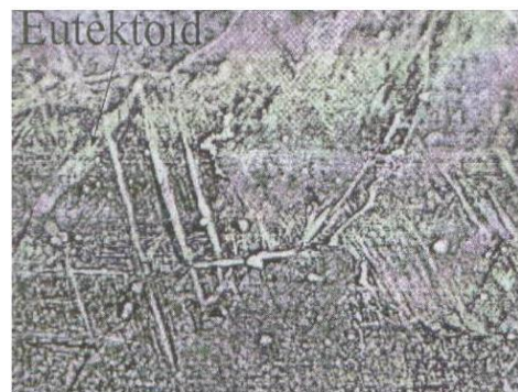
Figure 8 Microstructure of alloy quenched from 900°C and aged at 400°C for 1h (x960)
