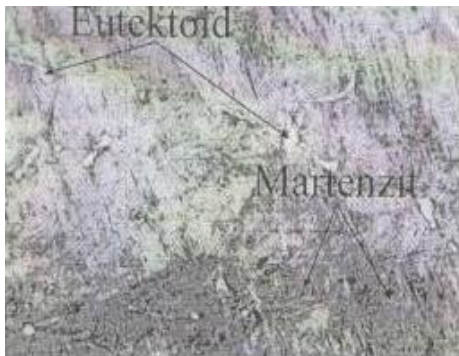
Figure 7 Microstructure of the alloy quenched from 850°C and aged at 400°C for 1h (x960)
