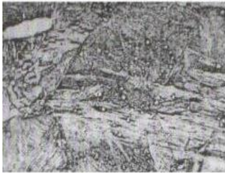
Figure 5 Microstructure of the alloy, annealed at 850°C for 10 min and water quenched (x960)
