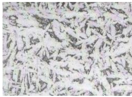
Figure 4 Microstructure of the alloy, hot deformed (x960)
