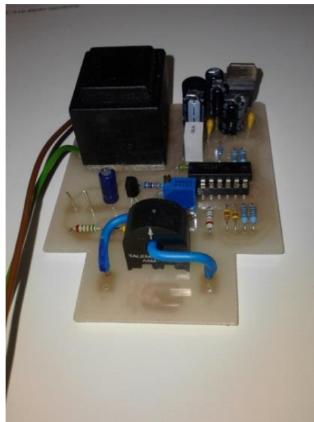
Figure 3 Single-sided transducer's PCB with the attached components
