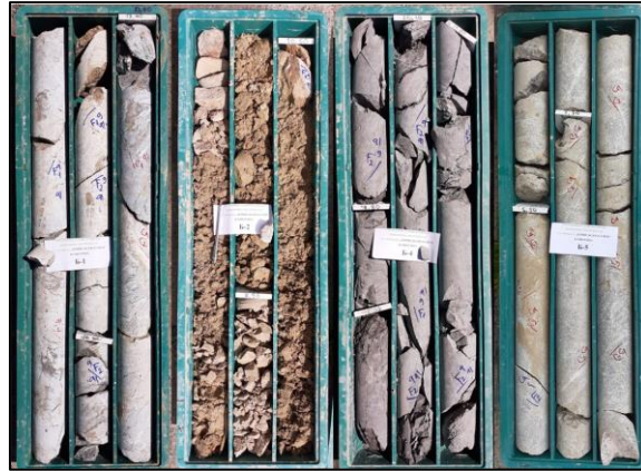
Figure 1 Marking core for geotechnical mapping
