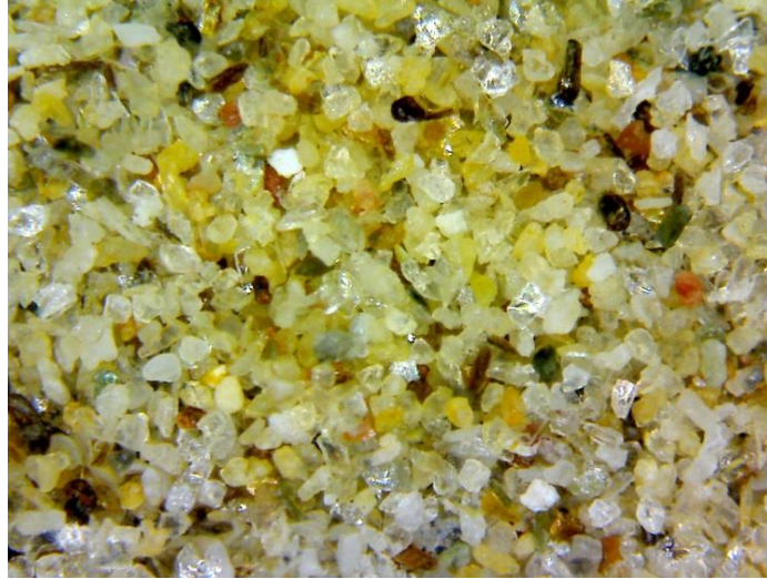
Figure 3 Microscopic appearance of fraction 0.250 / 0.125 mm, binocular magnification 40X
