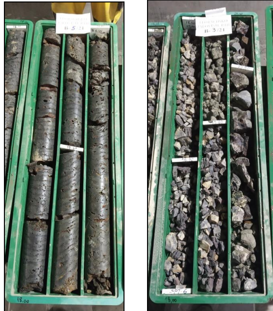
Figure 1 Smelter slag – Core from exploration drill-holes B-5/21 i B-3/21
