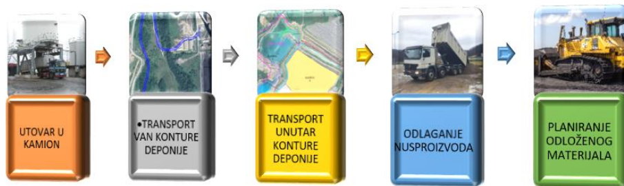
Figure 1 Technological process of loading, transport and disposal of by-products
