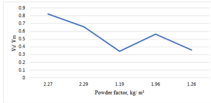
Figure 6 The ratio of ideal volume model and volume of the blasting model as a function of the applied powder factor
