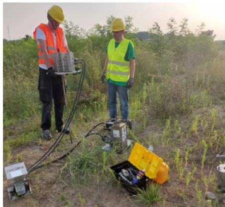
Figure 3 Dynamic penetrometer Pagani DPM 30/20 with dynamic penetration resistance curve q_d (MPa)
