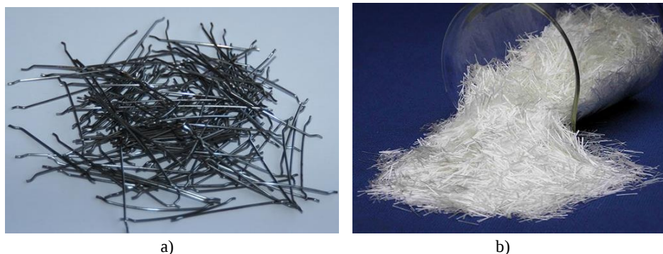
Figure 1 View of fibers: a) steel b) polypropylene
