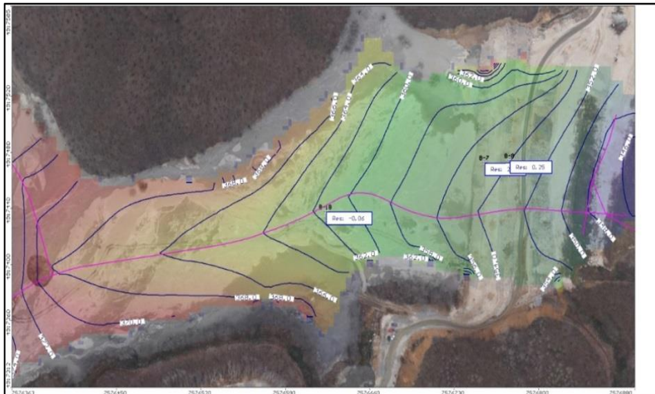
Figure 3 Map of hydroisohypsis and residual differences based on measurements from April 2024
