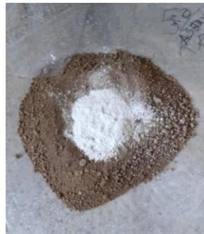
Figure 2 Homogenization material of subsoil with 5% lime
