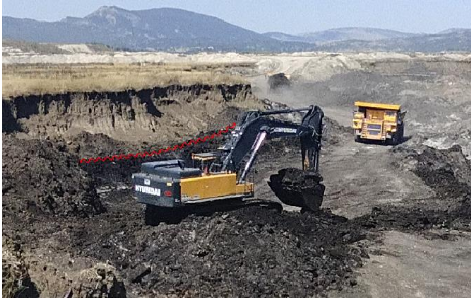
Figure 3 Contact of Quaternary sediments and roof clays and marls (red) with the transport path formed in the marls
