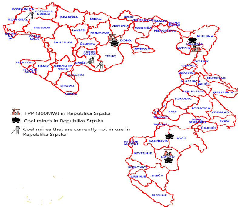
Figure 1 Spatial distribution of coal deposits and thermal power plants in Republika Srpska Source: Adapted from ERS and Znanje.org.
