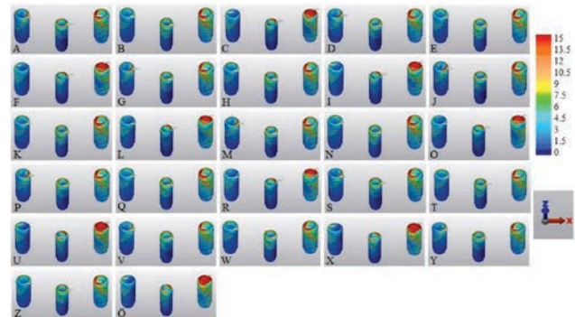
Figure 3. Von Mises stresses ( \sigma_{vM} ) on implants. A: Model 1, B: Model 2, C: Model 3, D: Model 4, E: Model 5, F: Model 6, G: Model 7, H: Model 8, I: Model 9, J: Model 10, K: Model 11, L: Model 12, M: Model 13, N: Model 14, O: Model 15, P: Model 16, Q: Model 17, R: Model 18, S: Model 19, T: Model 20, U: Model 21, V: Model 22, W: Model 23, X: Model 24, Y: Model 25, Z: Model 26, Ö: Model 27.
