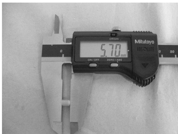
Figure 1. Mold for DOC testing according to ISO 4049 (shema) and digital caliper
