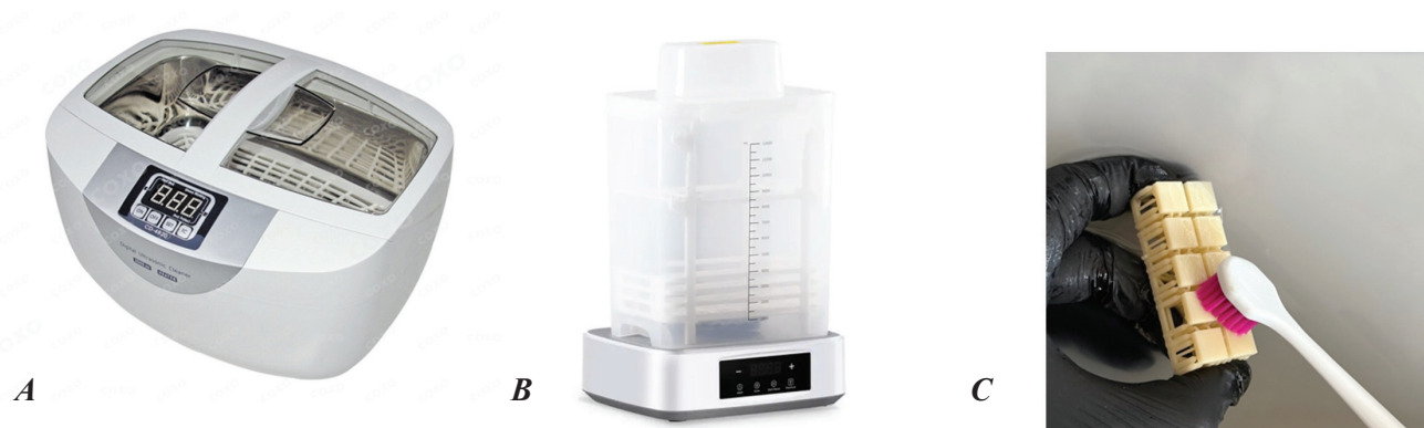
Figure 4. The three different equipment for rinsing methods: (A) Ultrasonic washer (B) Rotary washer and (C) Manual brushing method.
