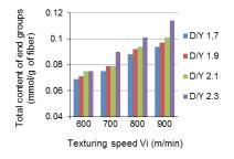
Figure 7. The dependence of the total content of end groups (mmol/g fiber) on D/Y ratio and the texturing speed Vi (m/min), at constant heater temperature of 210  $^{\circ}$ C
