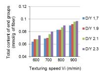
Figure 6. The dependence of the total content of end groups (mmol/g fiber) on D/Y ratio and the texturing speed Vi (m/min), at constant heater temperature of 200  $^{\circ}$ C
