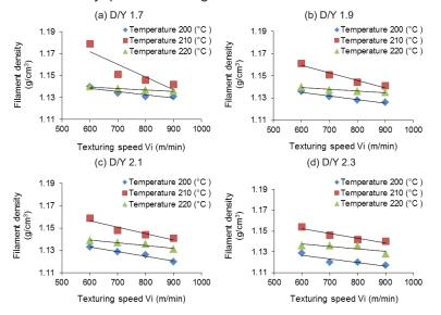
**Figure 1.** The dependence of filament density on the heater temperature T (°C) and the texturing speed Vi (m/min), at constant ratio of the surface disc speed to the linear yarn speed D/Y: a) 1.7, b) 1.9, c) 2.1, and d) 2.3.
