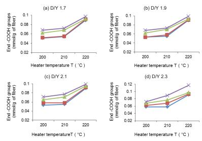
**Figure 5.** The dependence of -COOH end group content (mol/g fiber) on the heater temperature T (°C) and the texturing speed Vi (m/min) at constant ratio of the surface disc speed to the linear yarn speed D/Y of: a) 1.7, b) 1.9, c) 2.1 and d) 2.3.
