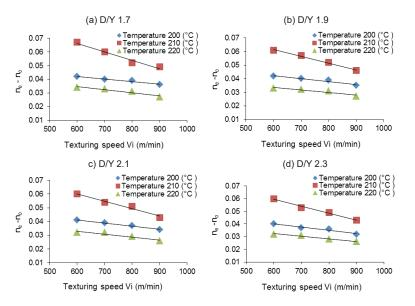
**Figure 3.** The dependence of double refraction, ne-no, on the heater temperature,  $T(^{\circ}C)$ , and texturing speed, Vi (m/min), at constant ratio of the surface disc speed to the linear yarn speed D/Y: a) 1.7, b) 1.9, c) 2.1, and d) 2.3.
