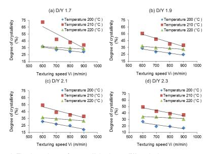
**Figure 2.** The dependence of a crystallinity degree (%) on the heater temperature T(°C) and the texturing speed Vi (m/min), at constant ratio of the surface disc speed to the linear yarn speed D/Y: a) 1.7, b) 1.9, c) 2.1, and d) 2.3.
