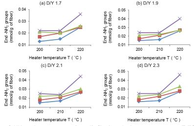
**Figure 4.** The dependence of  $-NH_2$  end group content (mmol/g fiber) on the heater temperature T (°C) and texturing speed Vi (m/min) at constant ratio of the surface disc speed to the linear yarn speed D/Y of: a) 1.7, b) 1.9, c) 2.1 and d) 2.3.
