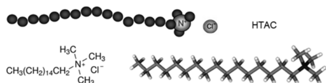
Figure 2. The molecular structure of hexadecyltrimethylammonium chloride ( \text{C}_{19}\text{H}_{42}\text{NCl} ) and 3D model of the cationic HTAC surfactant
