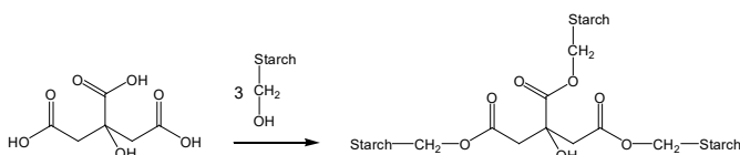
Figure 5. Possible structure of gel based on starch and citric acid
